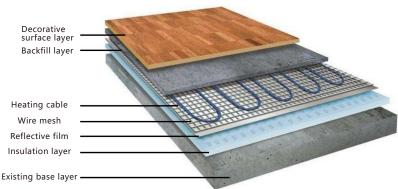
The product is mainly used for indoor floor heating and can be installed under tiles or floors to evenly transfer heat upwards by radiation, providing healthy and comfortable warmth.
