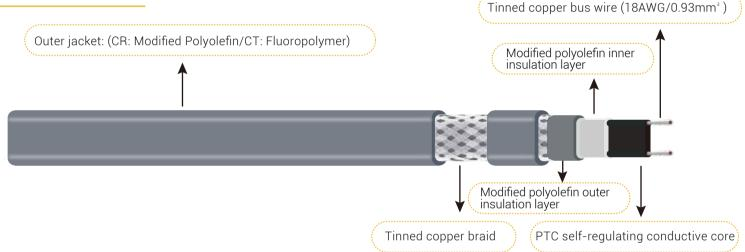
The extruded core tape, which made by parallel tinner copper bus wire and PTC semiconductor polymer heating material, and inner insulation layer of modified polyolefin are added to tinned copper braid and the outer jacket form a complete structure of SLL heating cable, in which the outer jacket can be made of modified polyolefin material (CR) or fluoropolymer material (CT) according to different application or area.
