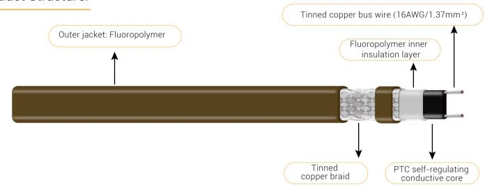
The extruded core tape, which made by parallel tinner copper bus wire and PTC semiconductor polymer heating material, and inner insulation layer of fluoropolymer are added to tinned copper braid and the outer jacket form a complete structure of HTP heating cable, in which the outer jacket can be made of fluoropolymer material (CT).
