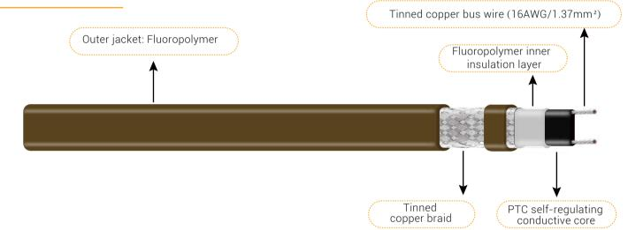
The extruded core tape, which made by parallel tinner copper bus wire and PTC semiconductor polymer heating material, and inner insulation layer of fluoropolymer are added to tinned copper braid and the outer jacket form a complete structure of HTP heating cable, in which the outer jacket can be made of fluoropolymer material (CT).
