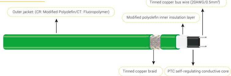
The extruded core tape, which made by parallel tinner copper bus wire and PTC semiconductor polymer heating material, and inner insulation layer of modified polyolefin are added to tinned copper braid and the outer jacket form a complete structure of HTM heating cable, in which the outer jacket can be made of modified polyolefin material (CR) or fluoropolymer material (CT) according to different application or area.
