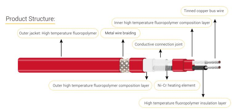
The main heating element for FCW heating cable is Ni-Cr heating conductor as above, which are connected to the bus wire sequencely via conductive connection joint as fixed length, this type of structure is to keep the stable power output consistently. Parallel conduct, core tape, and relative fluoropolymer insulation layer/composition layer are added to metal wire braiding and the outer fluoropolymer jacket form a complete structure of FCW heating cable.
