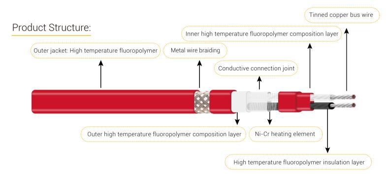
The main heating element for FCW heating cable is Ni-Cr heating conductor as above, which are connected to the bus wire sequencely via conductive connection joint as fixed length, this type of structure is to keep the stable power output consistently. Parallel conduct, core tape, and relative fluoropolymer insulation layer/composition layer are added to metal wire braiding and the outer fluoropolymer jacket form a complete structure of FCW heating cable.
